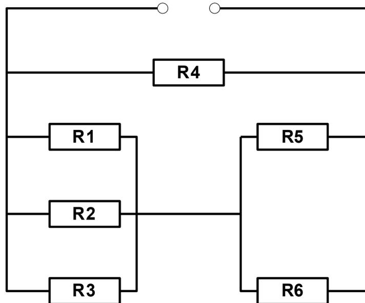
$$R_0 = 0,3 \text{ k}\Omega, R_1 = 20 \Omega, R_2 = 20 \text{ k}\Omega, R_3 = 40 \Omega, R_5 = 800 \Omega, R_6 = 1000 \Omega$$
