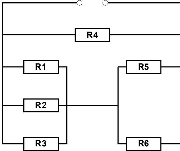
$$R_1 = 20 \Omega, R_2 = 20 \text{ k}\Omega, R_3 = 40 \Omega, R_4 = 0,5 \text{ k}\Omega, R_5 = 800 \Omega, R_6 = 1000 \Omega$$
